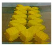
Model of **FLOATON**<sup>®</sup> BREAK WATER and the 1:1 scale prototype have passed laboratory and field tests successfully. Effective configuration to give maximum wave damping is given by the so-called 'slopingzigzag-holes' configuration.
